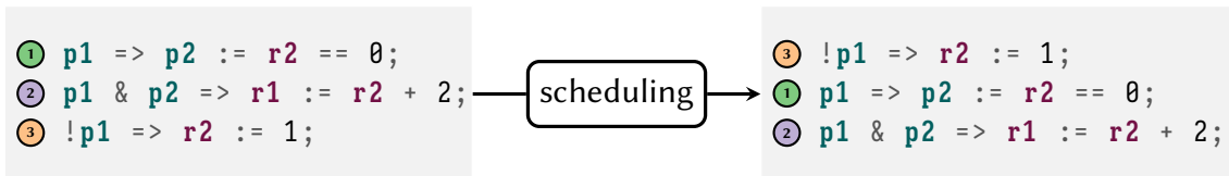
Figure 5.8: An example schedule. It is valid to move ③ before ① and ② because despite the appearance of data dependencies on r2 , ③ is in fact independent because its guard is mutually exclusive with the other two.
